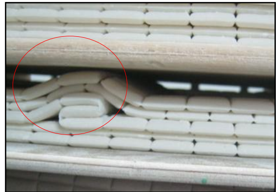
Gambar 4.13 Penyimpangan collecting sheet di Tray
